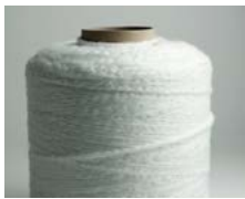
Sliver wound on the small cartoon tube with added twist (AT) (presentation D)
